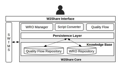
Figure 1. W2Share Software Architecture - workflow management is performed by the SWfMS.
